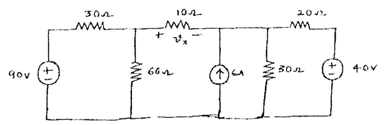
b) Compute the value of R that results in maximum power transfer to the  $10 \Omega$  resistor for the circuit shown below. Find also the maximum power. 8 M
