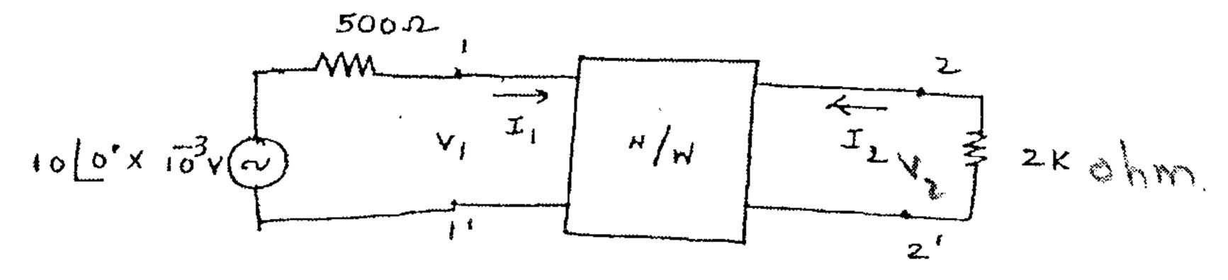
5. a) For the network shown, determine the transform impedance Z(s).
