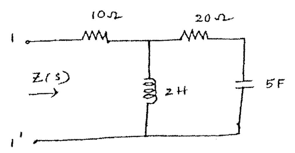
b) Find the driving point impedance of the network shown in the figure. Also find the zeros and poles of the network and locate the in the s-plane.
