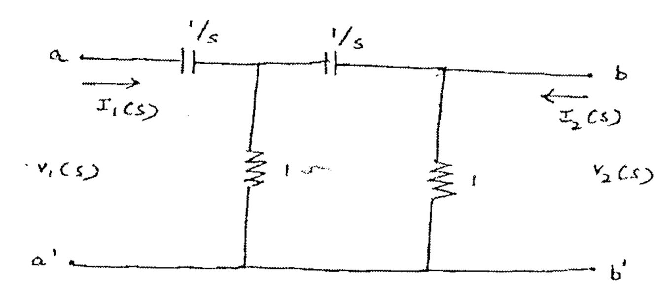
b) The hybrid parameters of a two port network shown in figure are  $h_{11}$ =0.003 $\Omega$ ;  $h_{12}$ = $h_{21}$ =100;  $h_{22}$ =50 $\mu$  mho. Find  $V_2$  and Z parameters of the network.
